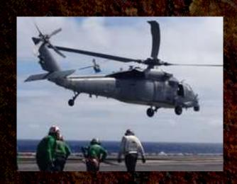
MH-60 chopper flying on 50-50 algae/ grease biofuel and petroleum fuel
